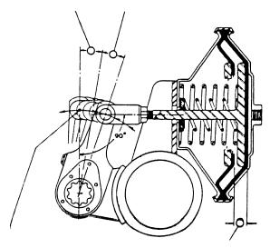
POINT OF GREATEST \*F LEVERAGE MOVEMENT PAST THIS POINT BRA RESULTS IN LESS LEVERAGE, M. REDUCED INPUT AND LOWER BRAKE EFFICIENCY.
